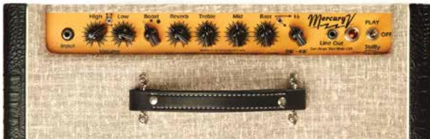
**The Mercury V's High and Low "channels" can be used separately or "jumpered" for added gain.**
