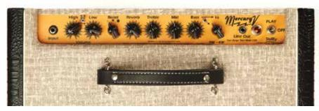
The Mercury V's High and Low "channels" can be used separately or "jumpered" for added gain.
